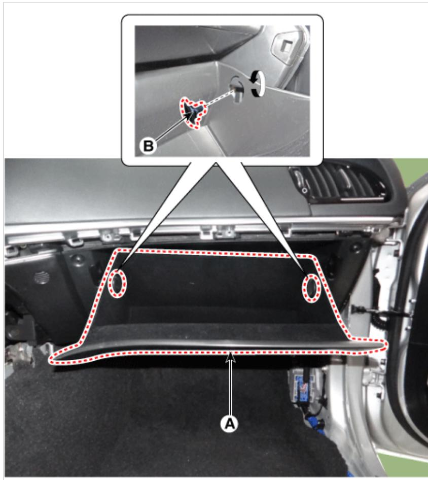
2. Remove the air damper (A) from the glove box (B).
