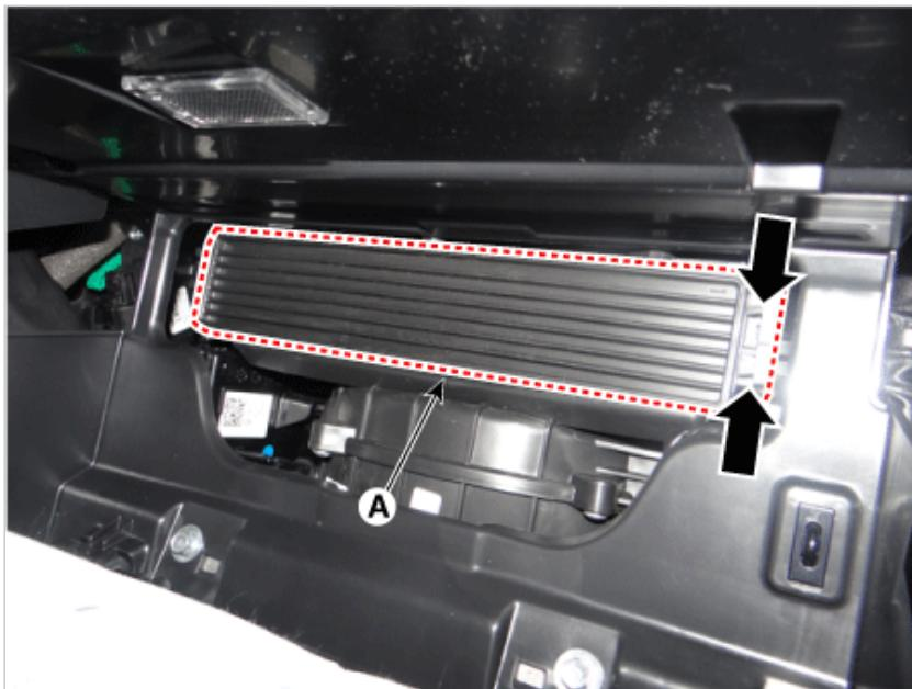
4. Replace the air filter (A) according to the replacement cycle on the user manual. When replacing it, mind the direction of the air filter.
